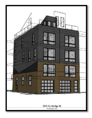
we worked with a structural engineer to add a steel package and concrete block wall down the middle to separate the homes so we could stack three more floors and build a rooftop deck for each home. Under this approach, we ultimately saved dramatically on the construction without having to demolish the structure, excavate for a foundation, and then pour a new foundation. We also didn't have to brick the side or rear of the home given the quality of the structure.
